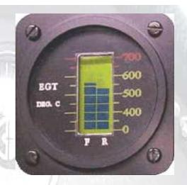
The Tasman dual EGT gauge combines the ease of reading of analog type displays with the advantages of digital technology. The temperatures of two exhausts can be read in the minimum of time, allowing more time looking outside the cockpit. The expanded scale gives the highest resolution to the temperature range of greatest importance. An alarm function flashes the display at a reading above 620 deg. to command the attention of the operator.
